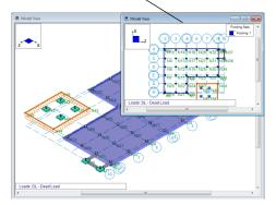
**Example 2**. Even though the original model view is rendered and in isometric view, the New Model View opens in wireframe, XZ Plan view (the RISAFoundation default view).
