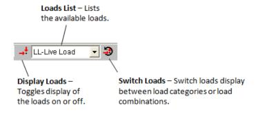
Experiment by "switching" to display load combinations (instead of categories):
