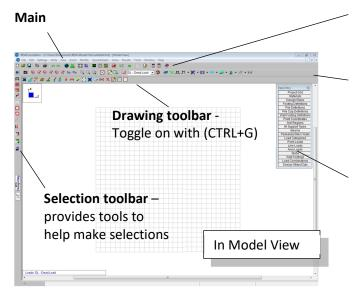
**RISA toolbar** – provides access to file operations, printing, changing design parameters, etc.
