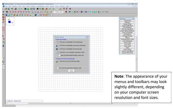
You have several startup options: you can choose to start drawing your model (either by defining beams or slabs, or using a template to generate it automatically), you can open an existing model, or you can click **Close** to work on your own.
