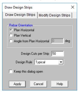
First, draw the strip to design the horizontal (Z axis direction) reinforcement.
