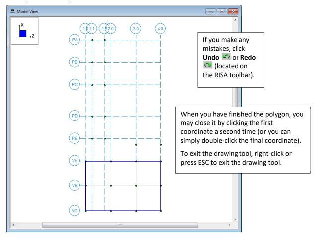
Next, create the slabs representing your combined footings over gridlines PB, PC, and PD. Rather than manually enter the drawing grid to create new snap points for drawing, you will import a DXF drawing grid.
