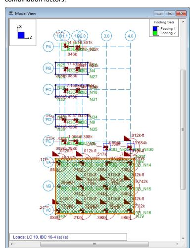
Using these tools, you will be able to view the displayed loads graphically, as multiplied by the load combination factors.
