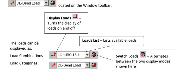
Experiment with these buttons by switching to display the load combinations:
