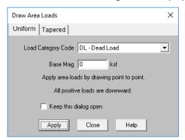
**Note:** Unlike RISA-3D, the positive vertical direction in RISAFoundation is assumed to be downward. Therefore, to apply a downward force, simply enter a positive magnitude.
