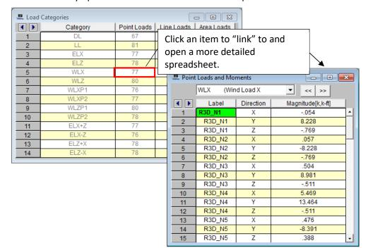
This automatically opens the **Point Loads- Wind Load X** spreadsheet:
