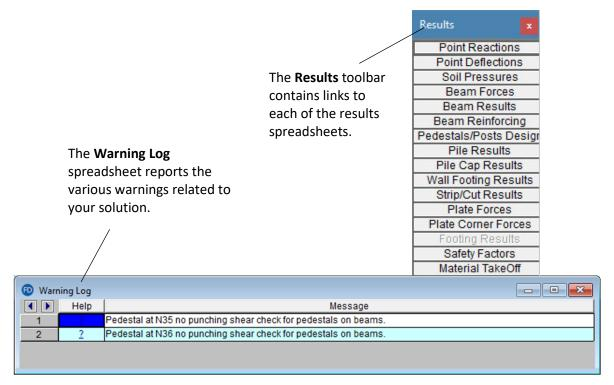
The two warnings associated with this model are in reference to a limitation in the pedestal design. These can be ignored because, while they limit the design checks performed by the program, they do not cause erroneous results in the design checks that were completed.
