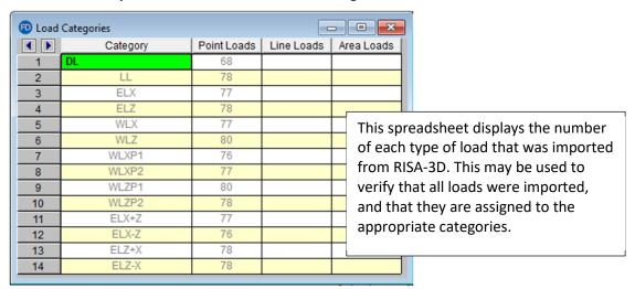
**Note:** All loads from RISA-3D import into RISAFoundation as unfactored point loads. In other words, the load magnitudes are independent of the load combination(s) run in RISA-3D, and they are sorted only by category. When solving in RISAFoundation, this allows you to apply the full load magnitude when running your foundation-specific load combinations.
