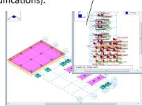
**Example 2**. Even though the original model view is rendered and in **XY view**, the **New Model View** opens in wireframe, isometric view (the RISAFoundation default view).
