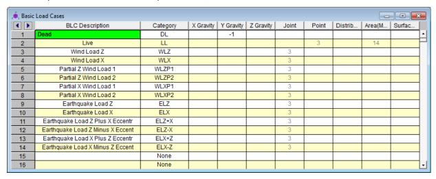
Notice that the dead, live, wind, and seismic load cases have been assigned to load categories (indicated by **DL, LL, WLZ**, **ELZ**, etc., in the **Category** column). All loads must have a load category assigned to them rather than **None**, or they will not transfer into RISAFoundation during the import process.
